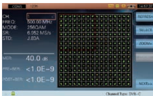
QAM constellation measurement
