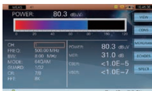
DVB-T signal measurement
